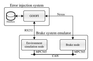
Figure 1. Experimental set-up.
