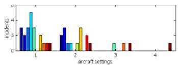
Number of incidents during ten simulations for different aircraft settings: aircraft settings 1 and 2 allow direction changes up to 5 degrees, while setting 3 and 4 allow direction changes up to 10 degrees; setting 2 and 4 approximate the position of neighboring aircraft by using also the most recent received messages.
