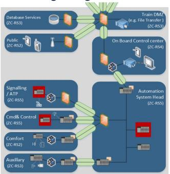
A common industrial practice is to keep same granularity and to assign a flat SL-T to each zone... E.g. on board equipment -> SL-T 3
