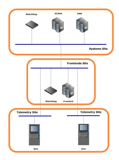
**Systems Site –** Higher layer of the architecture where the SCADA servers, the DMS and workstations are deployed.
