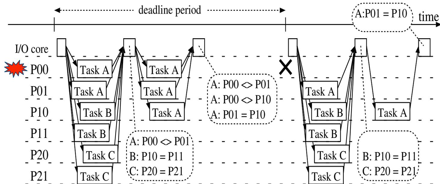
Tasks are redundantly loaded in several cores
