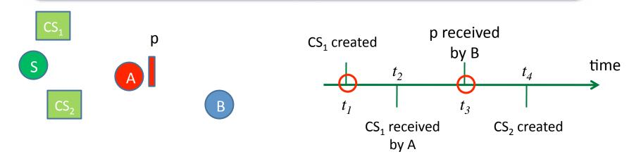
Packet p will be verified against CS<sub>2</sub> and not CS<sub>1</sub>. The attacker does not gain anything by observing CS<sub>1</sub>.
