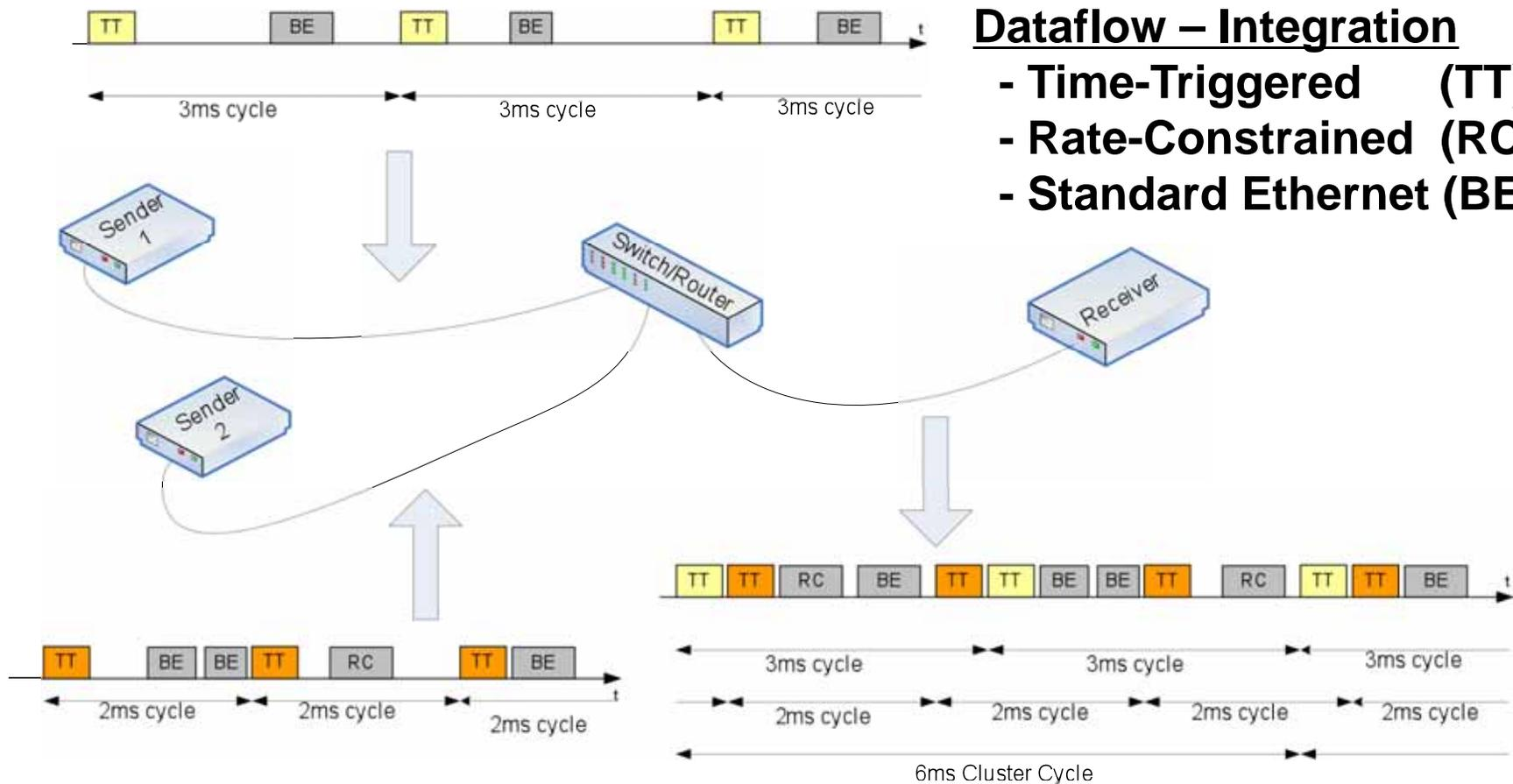
**TTEthernet Switch is also capable of changing traffic types, e.g. a message received as RC can be relayed as TT**
