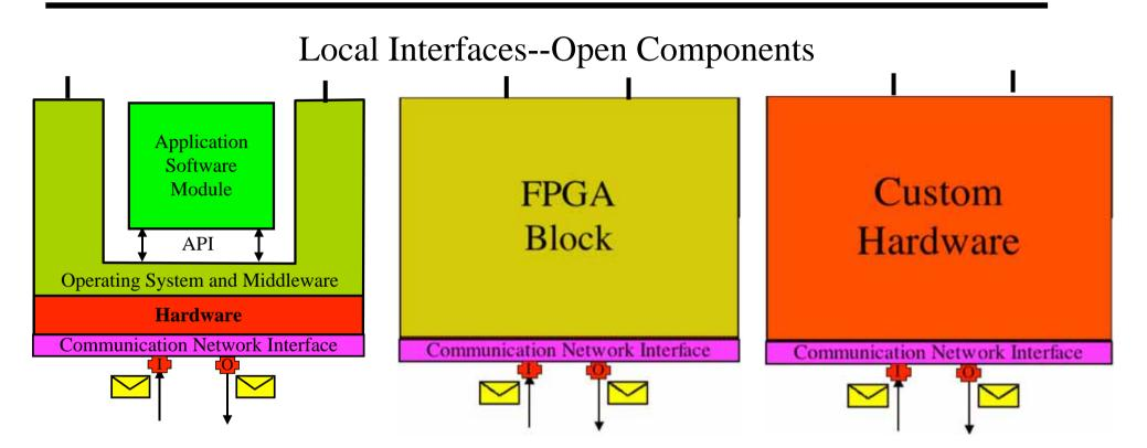
The Linking Interface (LIF) of all three different component implementations should have the same *syntax, timing* and *semantics*. For a user, it should not be discernible which type of component is behind the LIF.
