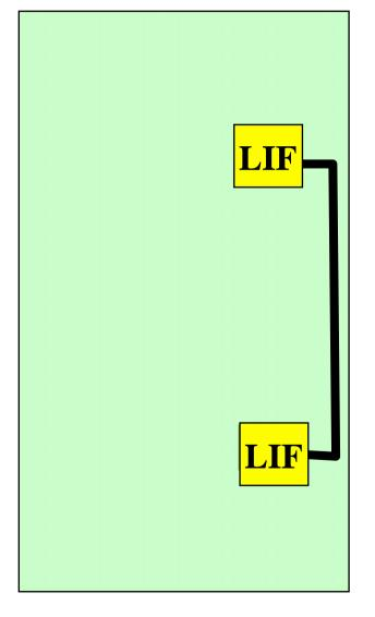
Chips are linked by *intra-device-level LIFs* to form a device.
