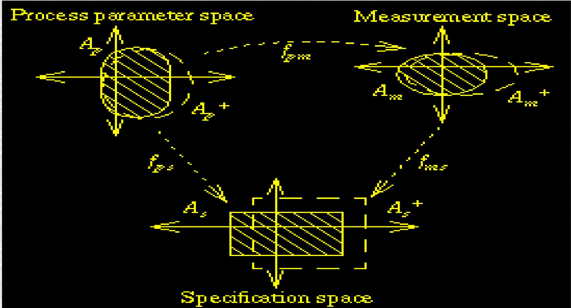
Mapping between measurement and specification spaces is derived using regression (MARS)
