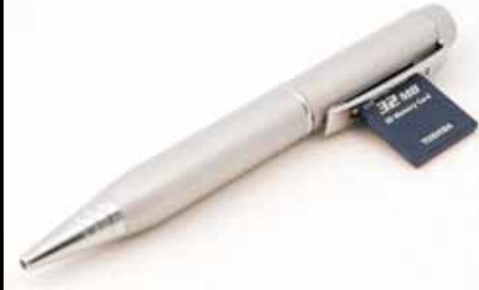
This functional pen not only has 128 MB of *storage* but also has a *USB connection* and a *connector* for SD memory cards.
